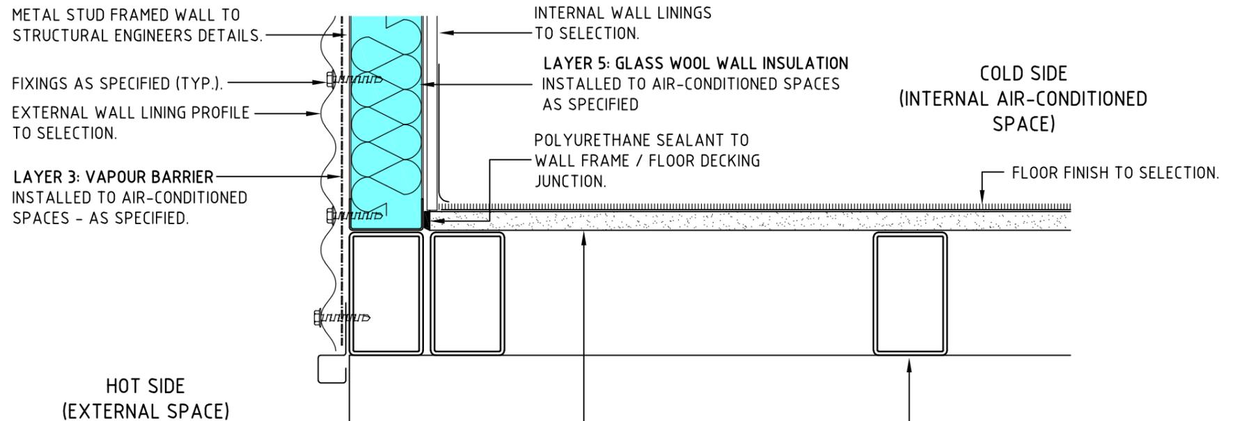
FIBRE CEMENT FLOOR DECKING FIXED AS PER MANUFACTURERS WRITTEN INSTRUCTIONS. PRIOR TO INSTALLATION FULLY PAINT UNDERSIDES OF EACH BOARD WITH CROMMELIN OR EQUIVALENT SEALER. ALL JOINTS IN DECKING TO BE SEALED WITH A POLYURETHANE SEALANT IN ACCORDANCE WITH THE MANUFACTURERS WRITTEN INSTRUCTIONS (TYP.).
