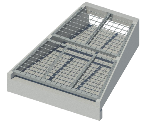
3D VISUALISATION - WINGWALL GRATE NOT TO SCALE
